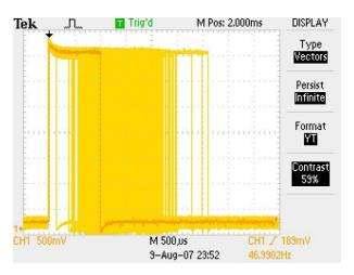
FIGURE 12: Jitter on 2.6.23-rc1 CON-FIG\_PREEMPT, P4
