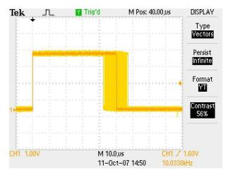
FIGURE 22: Jitter on RTLinux v3.2-rc1
