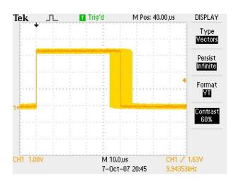
FIGURE 23: Jitter on RTAI v3.5
