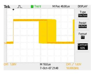
FIGURE 24: Jitter on LXRT (RTAI v3.5)
