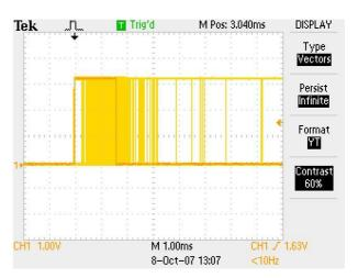
FIGURE 11: Jitter on 2.6.23-rc1 CON-FIG\_PREEMPT, VIA C3 600MHz
