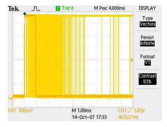
**FIGURE 10:** Jitter on 2.6.23-rc1 CON-FIG\_PREEMPT\_NONE, P4
