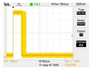
FIGURE 14: Jitter on 2.6.23-rc1-rt1 CONFIG\_PREEMPT\_RT, VIA C3 1GHz
