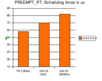
**FIGURE 25:** Scheduling times on P4 2.8GHz and VIA 1GHz, 600MHz for an rt thread demanding 50us
