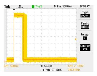
FIGURE 17: Jitter on 2.6.22.1-rt6 CON-FIG\_PREEMPT\_RT, VIA C3 1GHz
