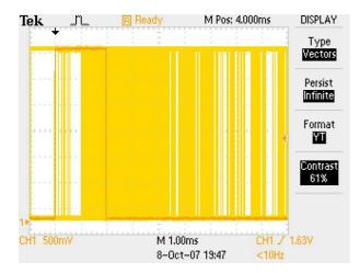
**FIGURE 9:** Jitter on 2.6.23-rc1 CON-FIG\_PREEMPT\_NONE, VIA C3 600MHz
