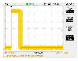
FIGURE 20: Jitter on 2.6.21.5-rt20 CON-FIG\_PREEMPT\_RT, VIA C3 1GHz
