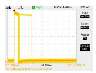
**FIGURE 21:** Jitter on 2.6.21.5-rt20 CON-FIG\_PREEMPT\_RT, P4
