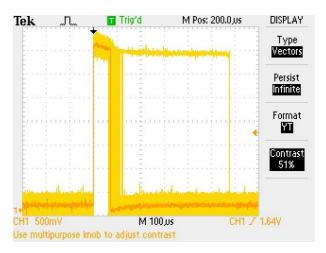
FIGURE 16: Jitter on 2.6.22.1-rt6 CON-FIG\_PREEMPT\_RT, VIA C3 600MHz
