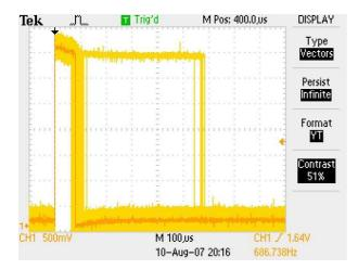
FIGURE 19: Jitter on 2.6.21.5-rt20 CON-FIG\_PREEMPT\_RT, VIA C3 600MHz
