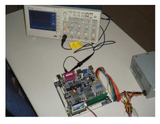
**FIGURE 1:** A Tektronix TDS 2014B Digital storage scope attached to a VIA C3 600MHz fanless board
