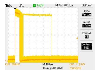
FIGURE 13: Jitter on 2.6.23-rc1-rt1 CONFIG\_PREEMPT\_RT, VIA C3 600MHz
